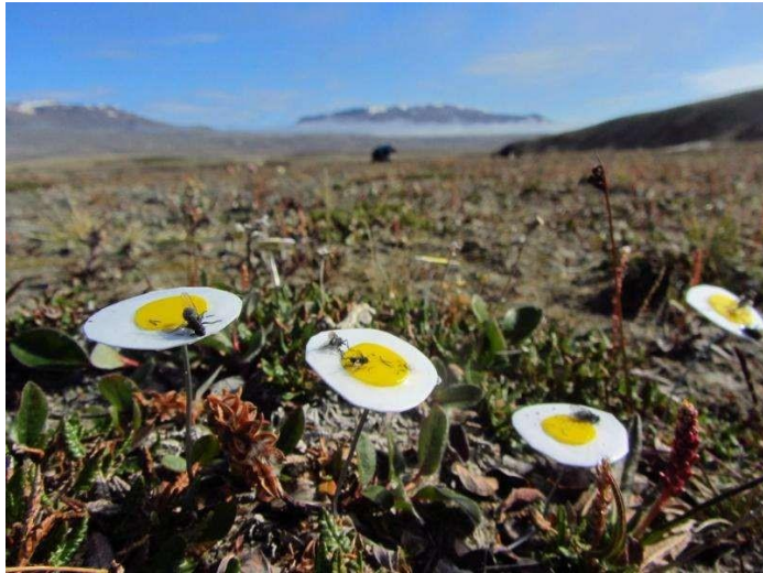
Fig 3: Although superficially resembling fried eggs, these sticky flower mimics were used to sample the insects visiting Mountain Avens ( Dryas ) Photo: Malin Ek
